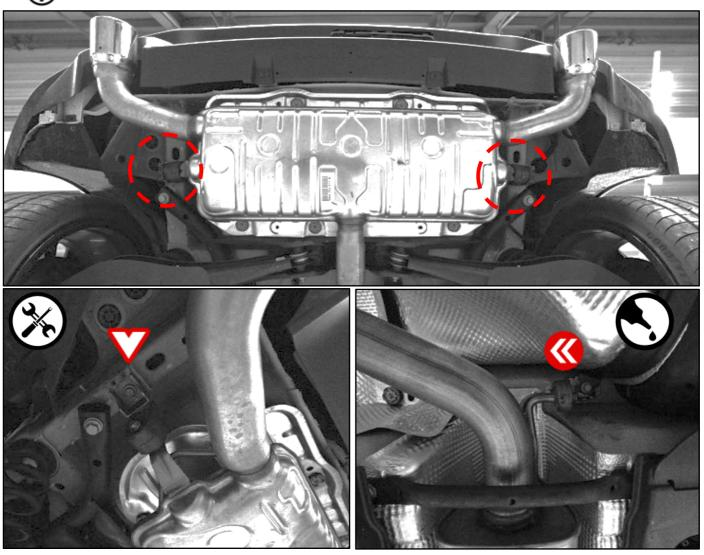
Loosen the clamp connection and remove the standard exhaust system.
