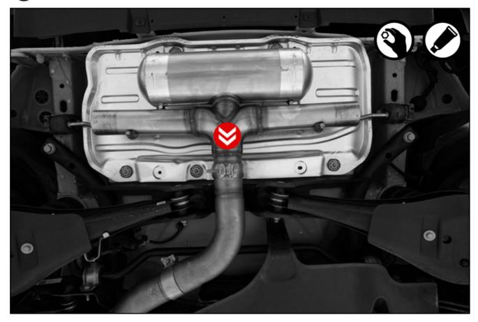
Remount the brackets onto the car chassis.
