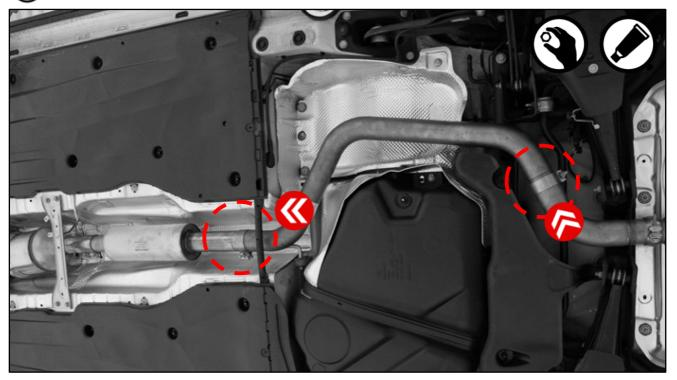
Remount the brackets onto the rubber hangers.
