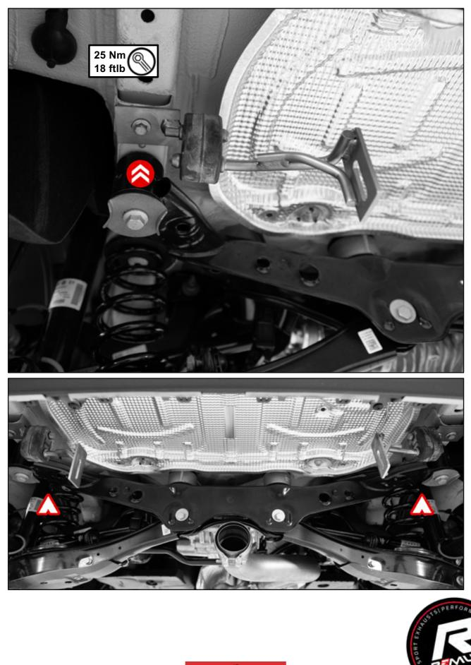
Dismount the stock chassis brackets and mount both REMUS brackets onto the same place.
